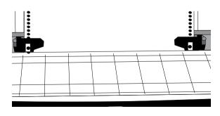
Remove the paper pieces, and use the platen knob to back 7. Replace the pull-up roller assembly, and close the access cover.
